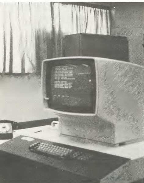
the video display unit installed for operator communication.
